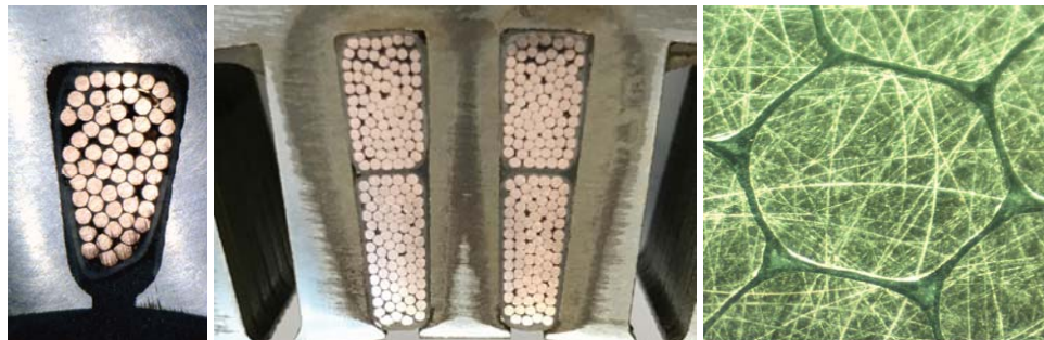
Figure 1: Classical Litz wire (left) and FLW (center) in stator slot and microscopic view of FLW (right)[2]
