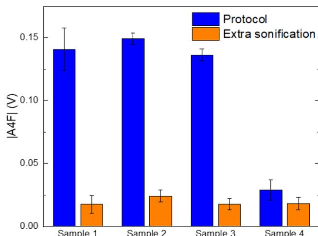
**Fig. 4.2. Effect of sonication on aggregation during protocol.** Background clustering for four samples with increasing number of sonication steps. Another measurement was done after an extra sonication step.
