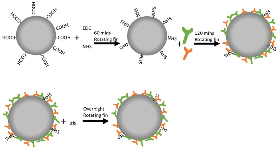
**Fig 3.1. Schematic view of particle functionalization.** Particles coated with carboxyl groups get activated by addition of EDC and NHS. After activation, primary amine groups on antibodies can bind on the activated sites. Remaining active sites get blocked by tris molecules to stabilize them.
