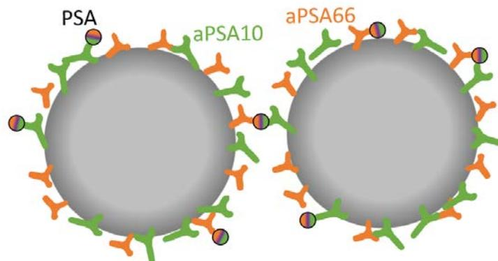
**Fig. 2.1. Schematic representation of a dimer in the antibody sandwich system.** Particles are covered with aPSA10 and aPSA66 antibodies. Each antibody binds only to one specific epitope on the PSA molecule.
