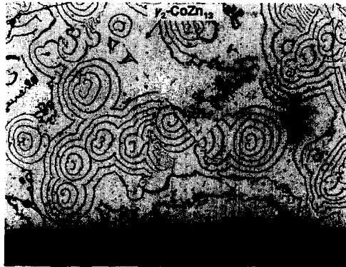
Figure 3. Cross-section of reaction layer perpendicular to the diffusion direction (BED).
