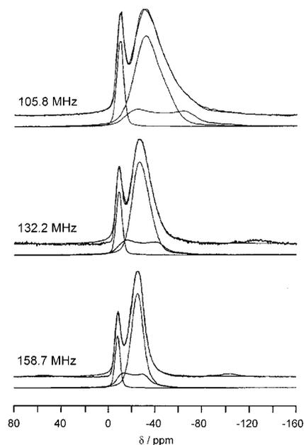
**Figure 5.**  $^{23}\text{Na}$  MAS NMR spectra and simulations (upper traces) for  $2\text{Mo}(\text{CO})_6/\text{NaY}$  and the individual components (lower traces) for the three indicated resonance frequencies.
