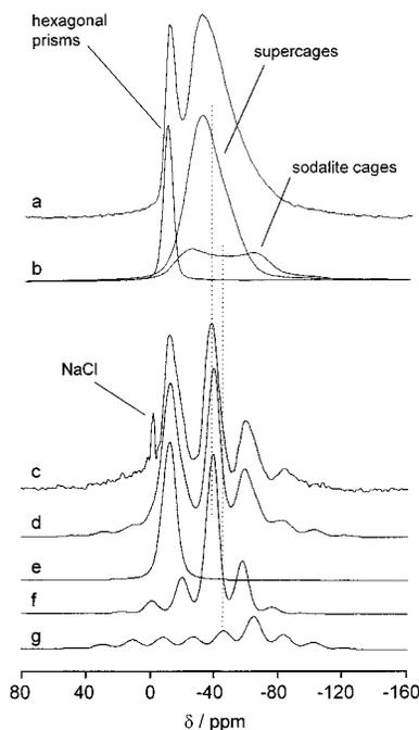
**Figure 4.** (a)  $^{23}\text{Na}$  MAS NMR spectrum of  $2\text{Mo}(\text{CO})_6/\text{NaY}$ ; (b) components of (a); (c)  $^{23}\text{Na}$  DOR NMR spectrum of  $2\text{Mo}(\text{CO})_6/\text{NaY}$ ; (d) simulation of components e–g, (e) Gaussian line at  $-9.9$  ppm; (f) quadrupolar component with  $\text{QCC} = 2.8$  MHz,  $\eta = 0.4$ , and  $\delta_{\text{iso}} = -19.7$  ppm; (g) quadrupolar component with  $\text{QCC} = 4.4$  MHz,  $\eta = 0.2$ , and  $\delta_{\text{iso}} = -1.6$  ppm.
