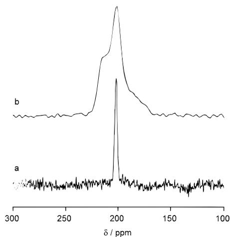
**Figure 9.** (a) Static  $^{13}\text{C}$  NMR spectrum of  $2\text{Mo}(\text{CO})_6/\text{NaY}$  and (b) static  $^{13}\text{C}$  cross-polarization (CP) NMR spectrum of  $2\text{Mo}(\text{CO})_6/\text{Na-NH}_4\text{-Y}$ .
