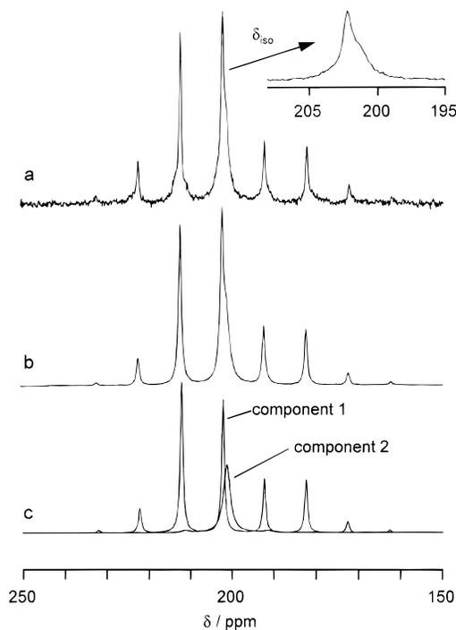
**Figure 11.** (a)  $^{13}\text{C}$  CPMAS NMR spectrum of  $2\text{Mo}(\text{CO})_6/\text{Na,NH}_4\text{-Y}$  at 293 K (spinning speed 1 kHz), (b) simulation of the spectrum, and (c) components of the simulation.
