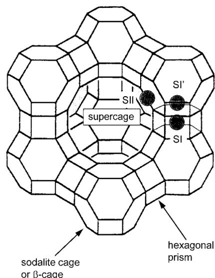
**Figure 1.** Cation positions in the structure of zeolite Y.
