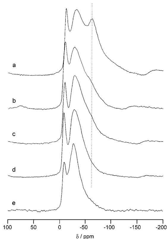
**Figure 3.**  $^{23}\text{Na}$  MAS NMR spectra of (a) dehydrated NaY, (b) a physical 1:1 mixture of dehydrated NaY and  $2\text{Mo}(\text{CO})_6/\text{NaY}$ , (c)  $1.4\text{Mo}(\text{CO})_6/\text{NaY}$ , (d)  $2\text{Mo}(\text{CO})_6/\text{NaY}$ , and (e) NaY saturated with  $\text{Mo}(\text{CO})_6$  in a helium flow.
