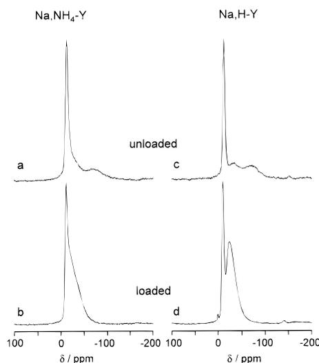
**Figure 8.**  $^{23}\text{Na}$  MAS NMR spectra of (a)  $\text{Na},\text{NH}_4\text{-Y}$ , (b)  $2\text{Mo}(\text{CO})_6/\text{Na},\text{NH}_4\text{-Y}$ , (c)  $\text{Na},\text{H-Y}$ , and (d)  $2\text{Mo}(\text{CO})_6/\text{Na},\text{H-Y}$ .
