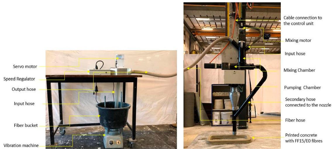
Figure 5. Shows the setup of the PAD system with PTS system.
