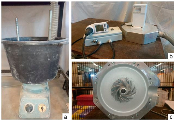
Figure 2. Various parts of the airborne PTS system, (a). Vibration bucket and Input hose , (b). Suction and blower chamber , (c) Rotor blade in blower chamber .
