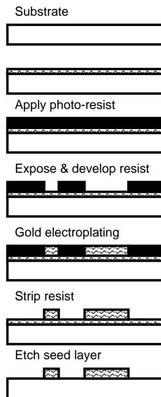
Figure 2- A schematic overview of the processing steps of electroplating.
