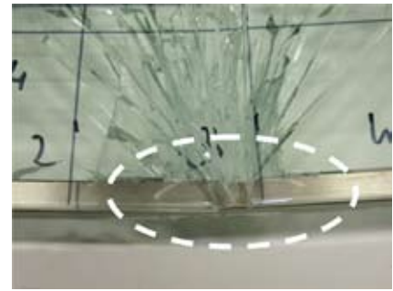
Figure 9: Delamination of the metal reinforcement at 60°C.
