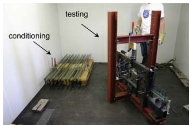
Figure 5: Climatic room at Ghent University. Conditioning and testing at 60°C within the same space.
