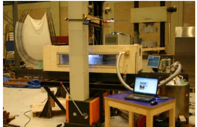
Figure 4: Bending test setup with a wooden climatic chamber, which has been cooled with vaporized liquid nitrogen to -20°C.
