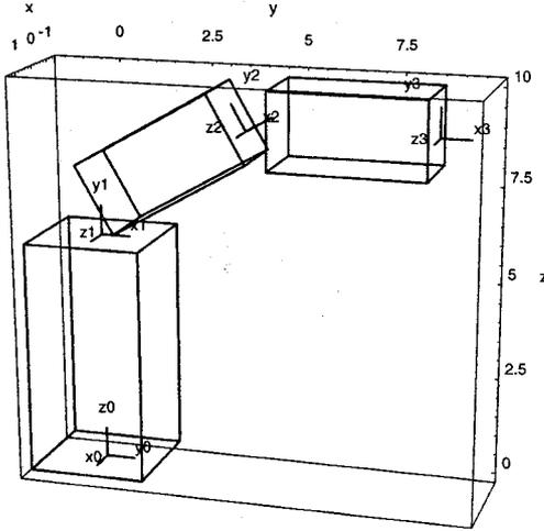
Figure 3: Orientation of the coordinate frames:  $O_0$  is placed at the center-base of link 1,  $O_i$  at the end of link  $i$ . The center of each servo motor (not shown) is located at  $O_0$ ,  $O_1$  and  $O_2$  parallel to the  $z$ -axis.
