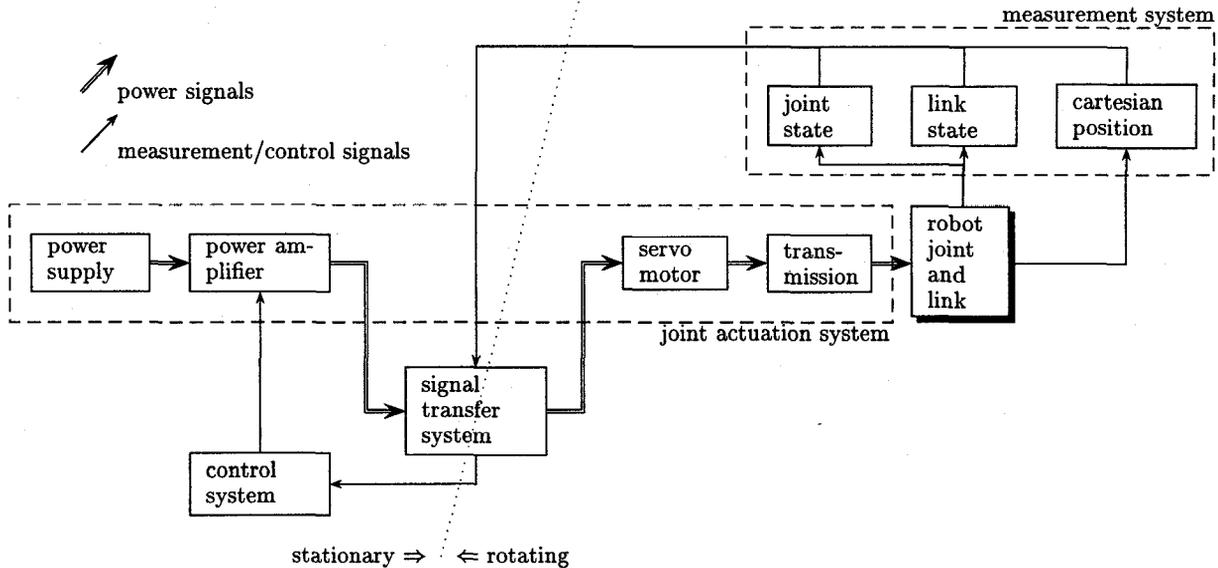
Figure 2: A possible functional lay-out for one of the RRR-robot's links; especially the position of the signal transfer system relative to the joint actuation system may vary (e.g., the power amplifier could also be placed on the rotating link, so right from the signal transfer system).
