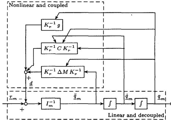
Figure 1: Block scheme of a rigid manipulator with transmissions.
