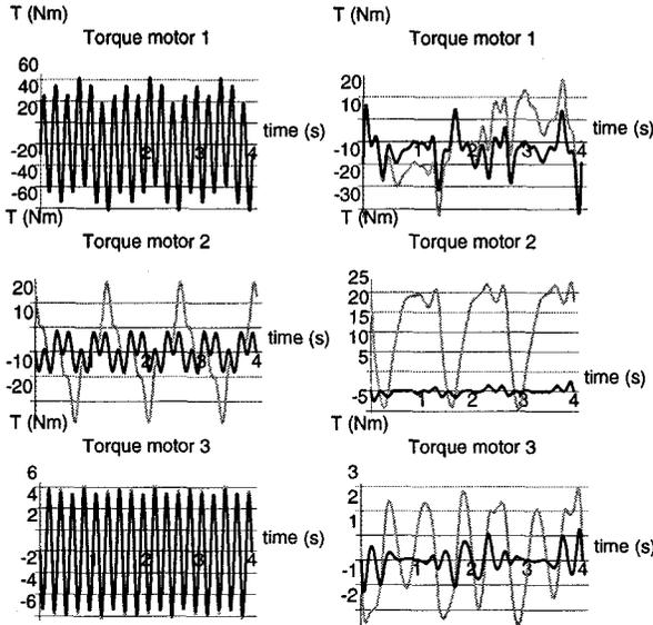
Figure 5: Required motor torques (thick gray lines) to realize a chosen motion pattern without accelerations (on the left) and with accelerations (on the right). The contribution of the Coriolis and centrifugal torques is shown with a thick black line.
