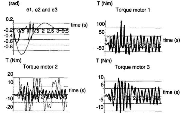
Figure 6: CTC controller: position errors  $e_1$  (thick gray line),  $e_2$  (thick black line) and  $e_3$  (thin black line); and motor torques (total torque with a thick gray line, contribution of Coriolis and centrifugal torques with a thick black line).
