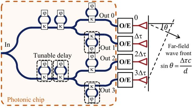
Fig. 2. Four-element linear PAA with optical TTD beamforming implemented by a photonic integrated chip based on a micro ring resonator tree structure.
