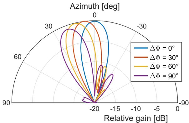
Fig. 8. Simulated beam steering in the horizontal plane at 85 GHz with the DRW antenna array, for increasing phase difference  $\Delta\Phi$  between adjacent antenna elements.
