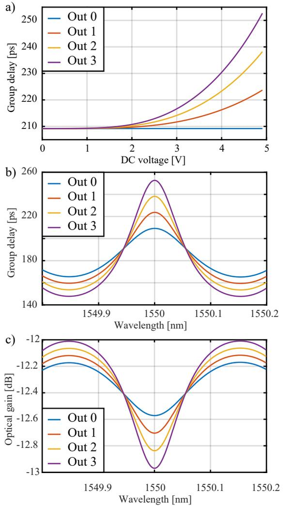
Fig. 3. Simulation results of integrated optical tree beamforming network: a) Maximum group delay at each output with respect to the DC voltage applied to the thermo-optic modulator, b) group delay with respect to the optical wavelength for an applied voltage of 4.9 V and c) optical gain with respect to the wavelength for an applied voltage of 4.9 V.
