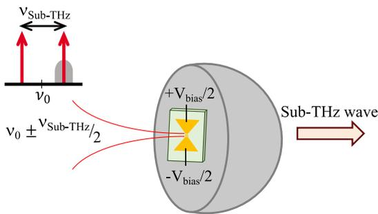
Fig. 4. Operating principle of bow tie photoconductive antenna with silicon lens for sub-terahertz communications.
