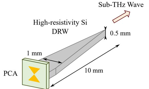
Fig. 5. Schematic drawing of a dielectric rod waveguide (DRW) integrated with a photoconductive antenna (PCA).
