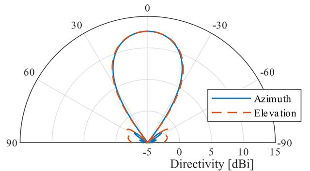
Fig. 6. Simulated radiation pattern at 85 GHz of a single DRW coupled to a photoconductive antenna.
