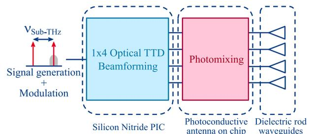
Fig. 1. Proposed system scheme to implement a sub-THz transmitter with beamforming capabilities, composed of three blocks: beamforming photonic integrated chip, photoconductive antennas and dielectric rod waveguide array.
