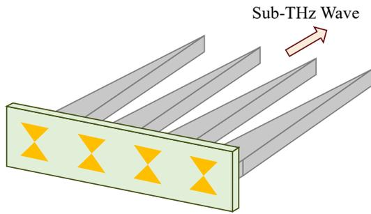
Fig. 7. Schematic drawing of a DRW antenna array integrated with four photomixers for sub-THz beam steering.
