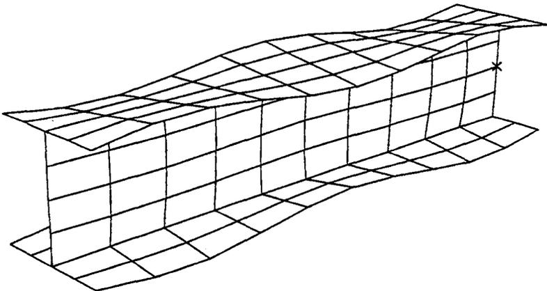
**FIG. 12. Buckling Mode of Uniformly Compressed I-Column**
