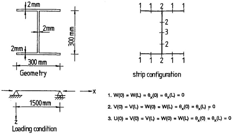
**FIG. 11. Geometry, Loading Condition, and Strip Configuration of I-Column**
