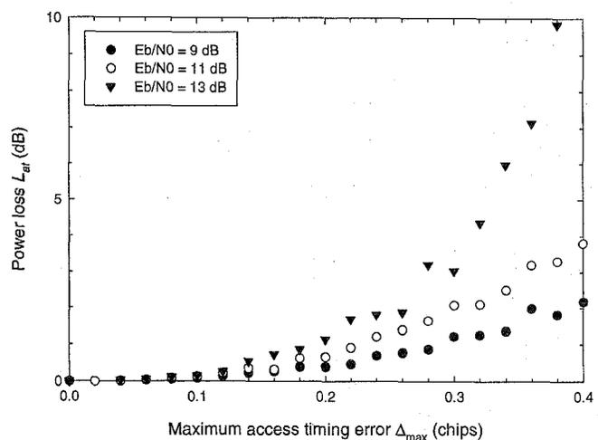
Fig. 4. Sensitivity of S-QPSK-CDMA to synchronization errors, for a BER of  $10^{-4}$  and for different values of the bit SNR  $E_b/N_0$ . The processing gain  $G_p = 18$  dB, and the number of active users  $N_u = 64$ .
