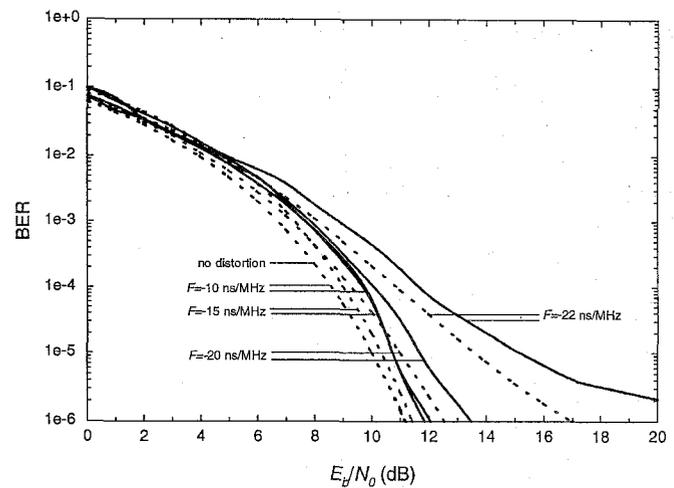
Fig. 11. System BER versus  $E_b/N_0$  for perfect (dashed) and imperfect (solid) chip timing and carrier recovery subsystems in a channel with linear group delay distortion.
