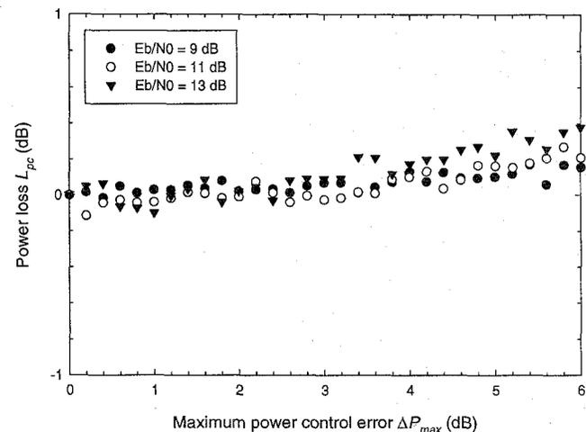
Fig. 5. Sensitivity of S-QPSK-CDMA to imperfect power control, for a BER of  $10^{-4}$  and for different values of the bit SNR  $E_b/N_0$ . The processing gain  $G_p = 18$  dB, the number of active users  $N_u = 64$ , and the maximum synchronization error  $\Delta_{max} = T_c/8$ .
