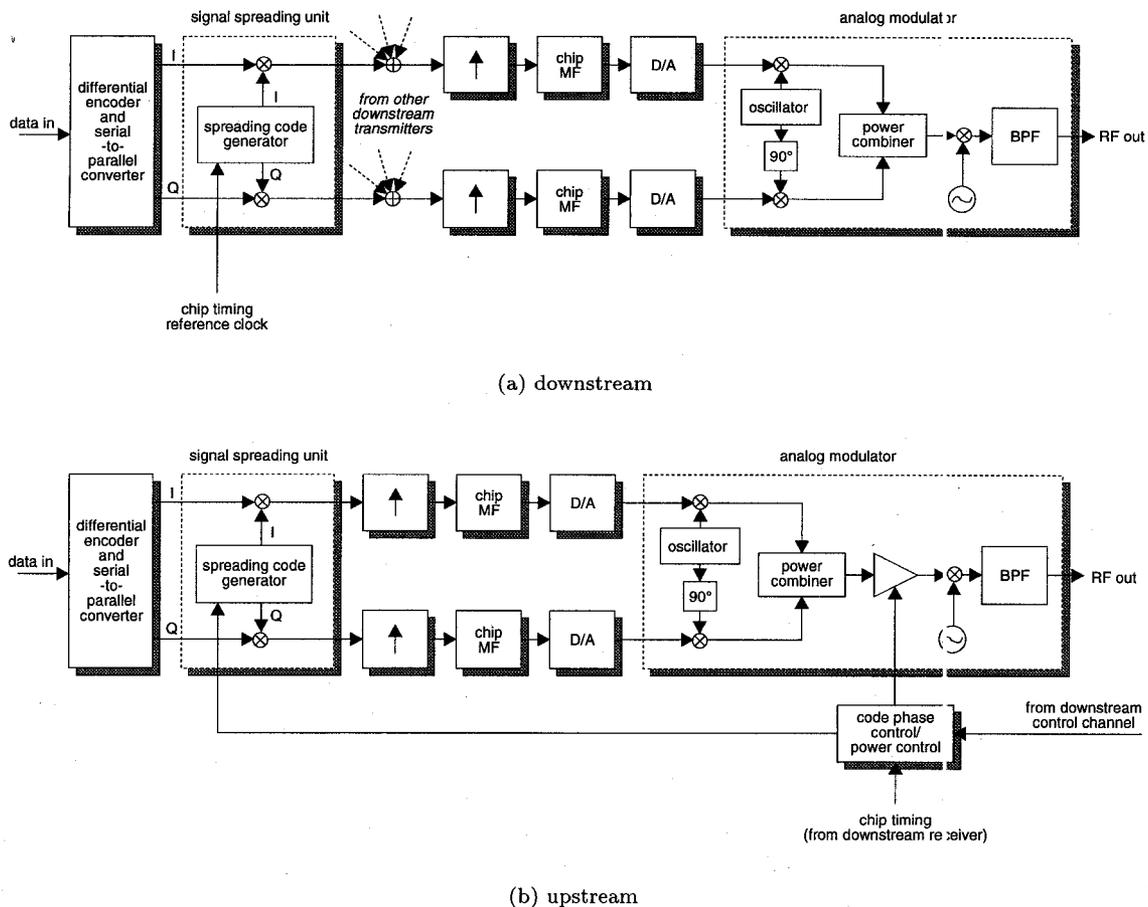
Fig. 6. Block diagrams of transmitters in an S-QPSK-CDMA system.
