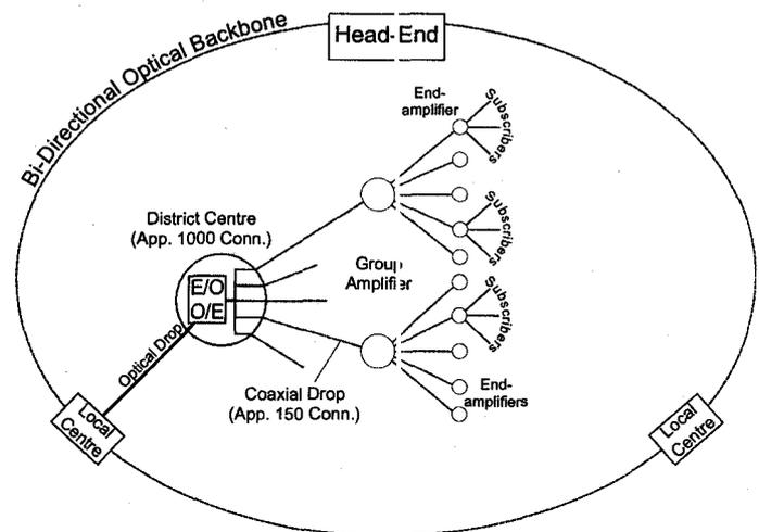
Fig. 1. Lay-out of a hybrid fiber-coax CATV network.
