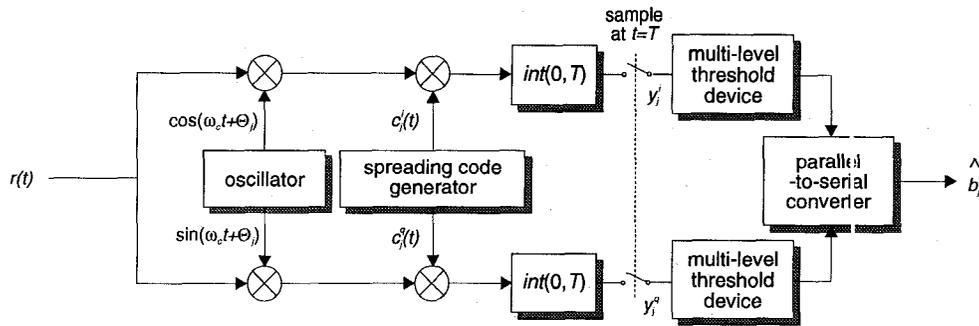
Fig. 2. Simplified model of an S-QAM-CDMA receiver.
