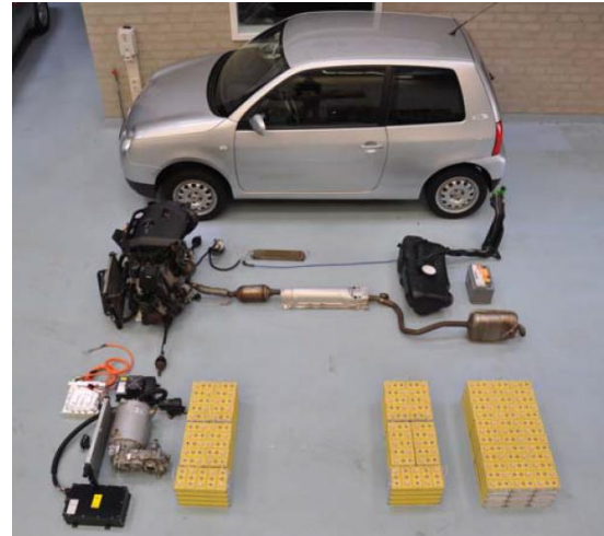
Figure 1: Lupo 3L with the existing diesel and new electric powertrain.
