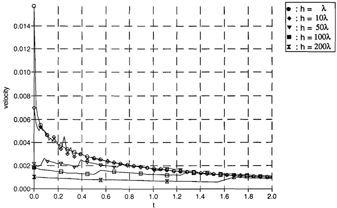
**Figure 8: contact line velocity as a function of the element size on the contact line.**
