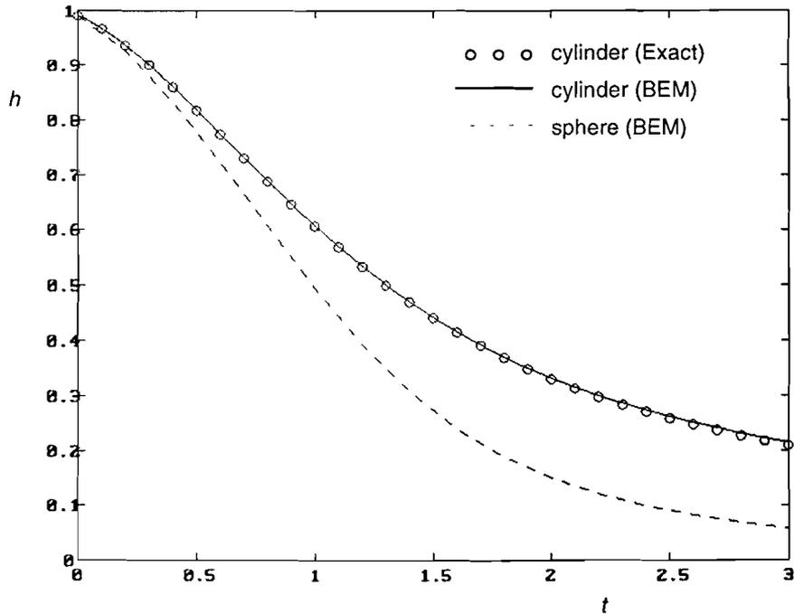
**Figure 1:** An excellent equivalence is obtained when the analytical (exact) height  $h$  of the coalescing cylinder is compared to the numerical solution. Moreover, the difference in the height development is compared to the coalescence of a sphere with the same initial radius.
