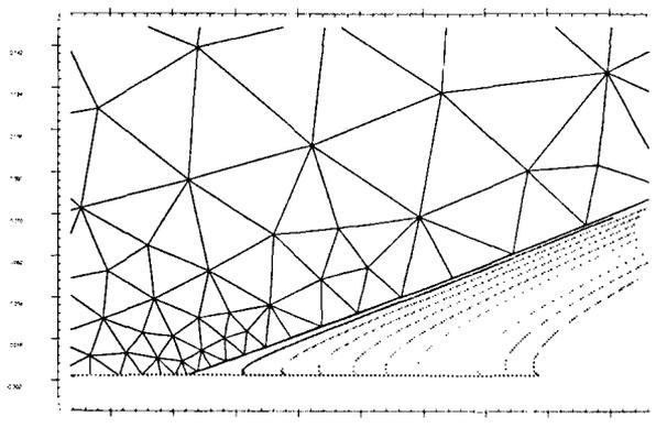
**Figure 6:** evolution of the surface near the contact line during 0.02 time units.
