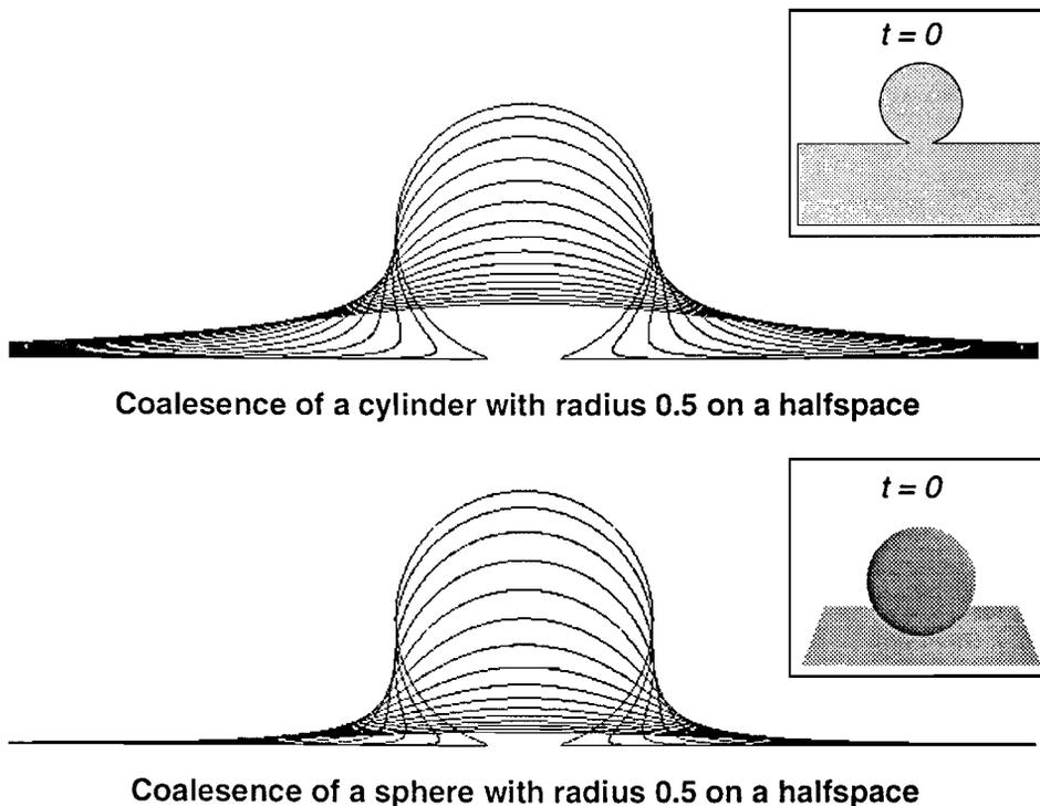
**Figure 2: A comparison between the coalescence of a cylinder on a plate and the coalescence of a sphere with both equal radius of 0.5 for  $t = 0.0(0.2)3.0$**
