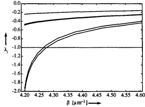
Fig. 3. Plot of the eigenvalues  $\lambda_j(\beta)$ ,  $j = 1, 2, 3, 4, 5$ , for a waveguide with rectangular cross section with edges of  $2 \mu\text{m} \times 1 \mu\text{m}$ . The guide is homogeneous and isotropic with refractive index 1.1, and the exterior region has refractive index 1.0. The wavelength in vacuo is  $1.5 \mu\text{m}$ . The mesh consisted of  $20 \times 10$  rectangles.
