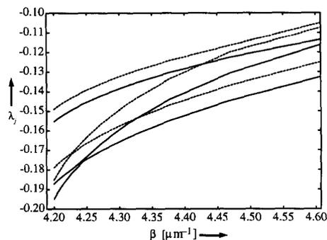
Fig. 6. Comparison of the third, fourth, and fifth eigenvalues as computed using a  $10 \times 10$  mesh (continuous curves) and a  $5 \times 5$  mesh (dashed curves). Physical parameters are as in Fig. 5.
