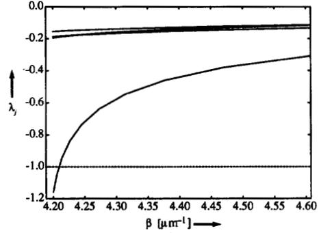
Fig. 5. Plot of the eigenvalues  $\lambda_j(\beta)$ ,  $j = 1, 2, 3, 4, 5$ , for a waveguide with square cross section with edges of  $1 \mu\text{m}$ . The guide is homogeneous and isotropic with refractive index 1.1, and the exterior region has refractive index 1.0. The wavelength in vacuo is  $1.5 \mu\text{m}$ . The mesh consisted of  $10 \times 10$  rectangles. Due to the symmetry, the smallest two eigenvalues coincide.
