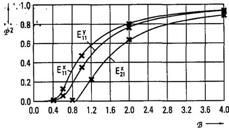
Fig. 8. Comparison of  $\mathcal{P}^2$  as a function of  $\mathcal{B}$  (see the text) of the smallest three modes of a rectangular waveguide of  $2 \mu\text{m} \times 1 \mu\text{m}$ , as computed by Goell and with the domain integral method. The mesh consists of  $30 \times 15$  rectangles.
