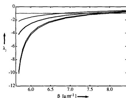
Fig. 7. The smallest five eigenvalues as functions of  $\beta$  for a rectangular waveguide of  $2 \mu\text{m} \times 1 \mu\text{m}$  and refractive index 1.5. The exterior region has refractive index 1.0, the wavelength in vacuo is  $1.118 \mu\text{m}$ . A  $5 \times 10$  mesh was used. The third and fourth eigenvalues are almost identical and overlap in the figure.
