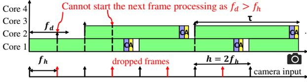
Fig. 4: Illustration of inter-frame dependencies with  $f_d > f_h$ . Note: 1) Even if more cores are available they cannot be used due to inter-frame dependencies; 2) Our method as compared to [7] does not restrict  $\tau$  to be an integral multiple of  $f_h$ ; 3) If  $f_d \leq f_h$  then  $h = f_h$  using all four processing cores.
