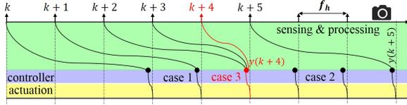
Fig. 5: Illustration of cases described in Section IV-B. The samples  $k + 3$  and  $k + 4$  have lower workloads and thus the latest output measurement  $y(k + 4)$  is available within one  $f_h$ . Note that for case 2, the latest measurements are not available and thus  $u(k + i)$  is computed based on the MPC prediction model.
