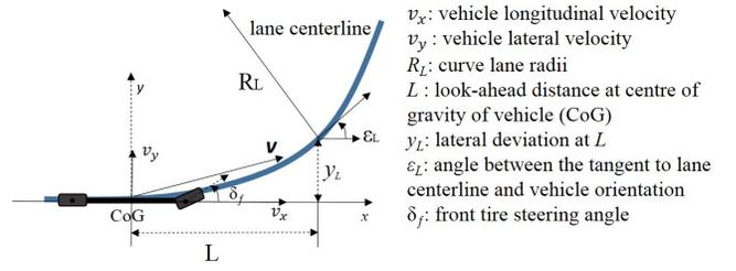
Fig. 6: Vision-based lateral control system derived from [15].
