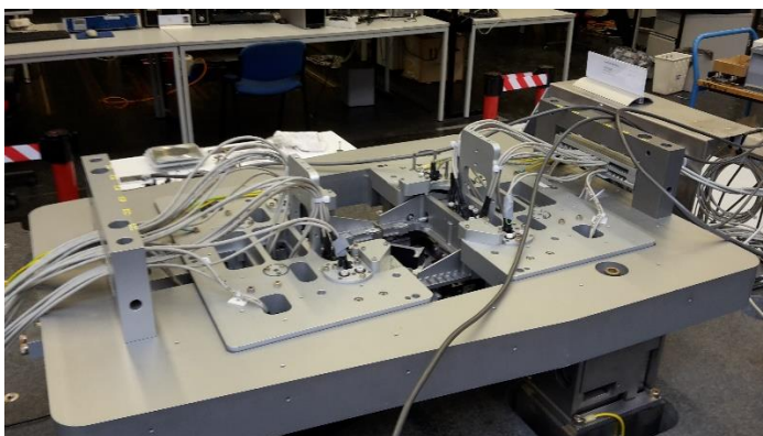
(a) Free floating reticle stage.
