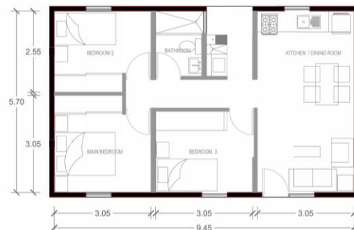
Figure 2: Floorplan of the house prototype
