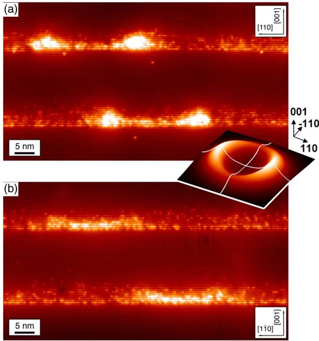
FIG. 4. (Color online) Filled states topography image of a cleaved QR in the  $(1\bar{1}0)$  plane (a) and  $(110)$  plane (b),  $V_{\text{sample}} = -3$  V. The height scale is 0 nm (dark) to 0.25 nm (bright). The inset shows the modeled QR.
