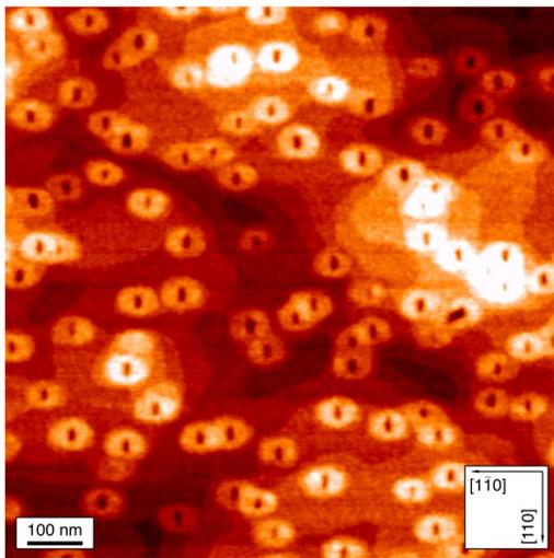
FIG. 1. (Color online)  $1 \times 1 \mu\text{m}^2$  atomic force microscopy image showing the anisotropic distribution of InAs/GaAs dot material after 2 nm GaAs capping and 1 min annealing at growth temperature under  $\text{As}_2$  flux. The height scale is 0 (dark) to 2.5 nm (bright). The height of the ring-shaped islands is about 1 nm. Atomic steps can be seen in the image.
