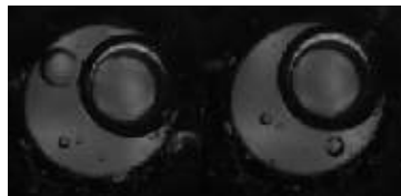
(c) To identify bubbles with a minimum bubble diameter of 400\mu m . The bubble coalesce multiple time before it leaves the electrode hole.
