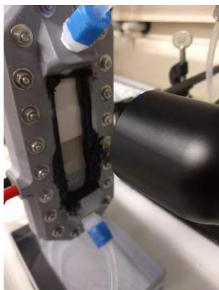
(a) Design of the 3D printed electrochemical cell.
