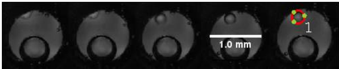
(a) To identify bubbles with a bubble diameter between 200 and 300\mu m . In the left the bubble is partly visible behind the electrode. A few frames later the bubble goes to the hole as shown in the right.
