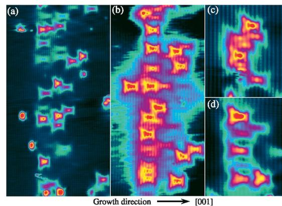
FIG. 1 (color). X-STM constant-current images of Mn  $\delta$ -doped GaAs with intentional Mn concentrations of  $3 \times 10^{13} \text{ cm}^{-2}$ : (a)  $51 \times 29 \text{ nm}^2$ ; (b)  $43 \times 20 \text{ nm}^2$ ; (c)  $12 \times 10 \text{ nm}^2$ ; (d)  $13 \times 10 \text{ nm}^2$ . Images were acquired at a sample bias of  $U_s = +1.5 \text{ V}$  on a cleaved (110) surface. Note appearance of continuous background DOS around the layer in (b).
