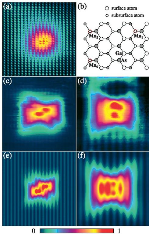
FIG. 2 (color). Topography of Mn-Mn pairs: (a)  $12 \times 12 \text{ nm}^2$ , X-STM image of two ionized Mn separated by 1.4 nm ( $U_s = -0.6$  V); (b) schematic of the (110) surface showing the location of subsurface Mn; (c) same area as (a), imaged with  $U_s = +1.1$  V so the Mn are neutral; (d)  $6 \times 6 \text{ nm}^2$ , X-STM image of two Mn separated by 0.8 nm ( $U_s = +1.55$  V); (e), (f) calculation with TBM of (c), (d), with parallel spins.
