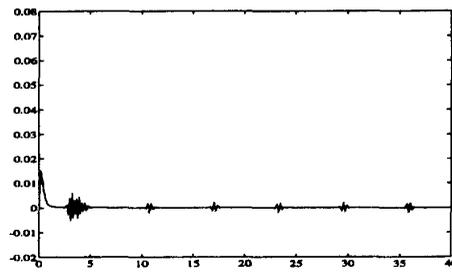
Figure 2: The output  $y_2$  of the system  $\Sigma_q$  in closed loop with the linear static state feedback (46).
