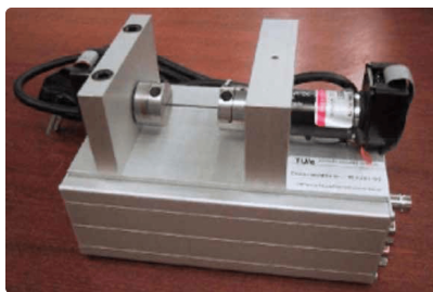
Figure 1.1: A Mass-Spring-Damper system, i.e. the PATO setup at the TU/e.
