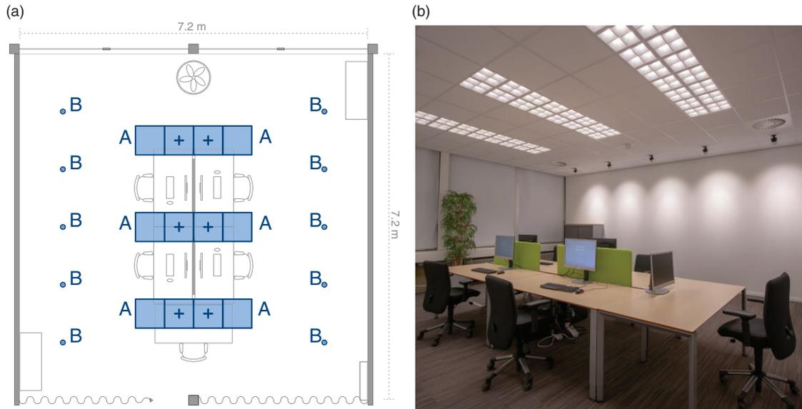
**Figure 1.** Layout and impression of the experimental setup – luminaire type A: general lighting luminaires, '+' indicates the added luminaires of the same type compared to de Vries *et al.*<sup>21</sup> Luminaire type B: Spots
