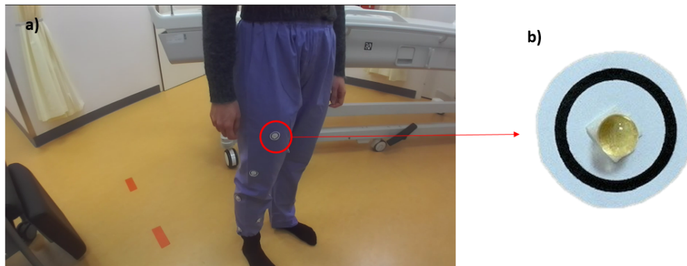
Figure 1. a) Marker position on the subject leg to be visible on the MR and video acquisitions. b) Magnified view on the marker employed to achieve visual tracking.
