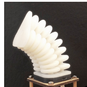
Fig. 1. Soft robot manipulator module entirely 3D-printed from a soft and flexible polyamide material.
