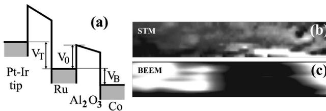
FIG. 1. (a) Energy diagram of the studied system; STM (b) and BEEM (c) images of the junction area of  $160\text{ nm} \times 17\text{ nm}$ .
