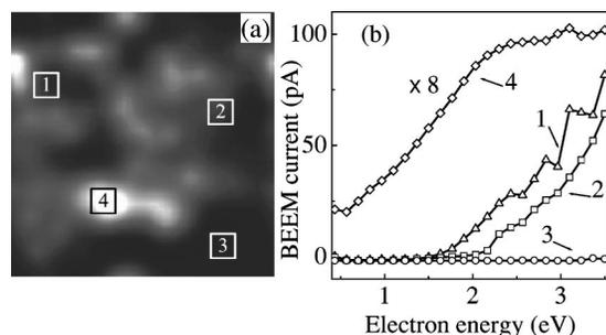
FIG. 3. (a) Spatial variation of transmission of the tunnel junction at 2 eV. Scanning area is  $510\text{ nm} \times 510\text{ nm}$ . (b) Spectroscopy curves corresponding to the marked areas of the left panel.
