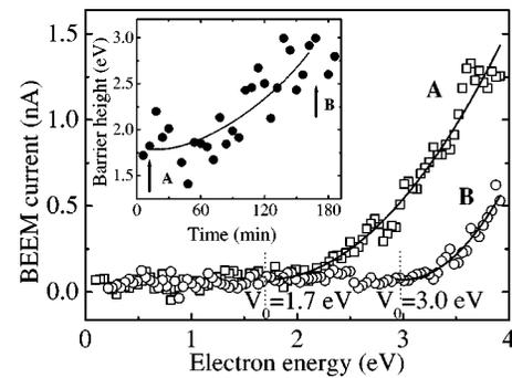
FIG. 2. Dependence of the transparency on the electron energy. (curve A) at the start of the measurement series; (curve B) after 3 h of current injection. Continuous curves represent a fits with power 2 law. The inset represents the evolution of the barrier height in time; the curve in the inset is a guide to the eye only. Arrows A and B mark the points corresponding to the curves A and B.
