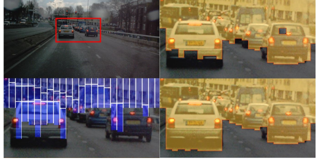
Figure 3. Results under low-light conditions: the brightened left camera image with a region of interest (top left), the results of [3] with partially undetected cars (bottom left), our color-only result (top right) and our distance-aware color-only result (bottom right).
