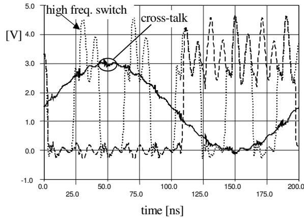
Figure 2: Transient simulation results on the test PCB.
