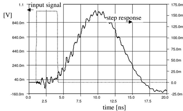
Figure 4: Results step-response simulation on LC-filter.
