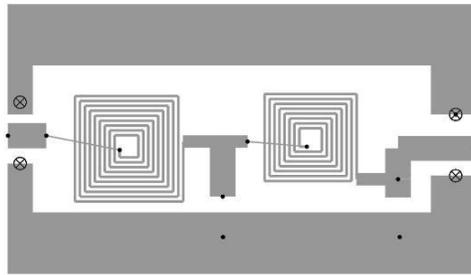
Figure 3: Double LC-filter layout structure.
