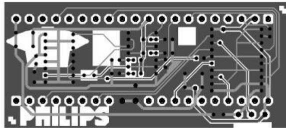
Figure 1: Layout of a 2-layer test PCB.
