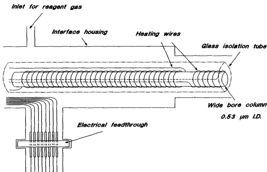
Fig. 1. Schematic diagram of the laboratory-made SFC-MS interface.
