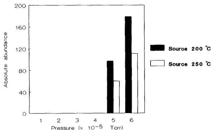
Fig. 3. Abundance of the protonated molecular ion of Tinuvin 770 as a function of the reagent gas pressure in the mass analyser. The ion source was held at 200 and 250°C, respectively. Other experimental conditions as in Fig. 2.
