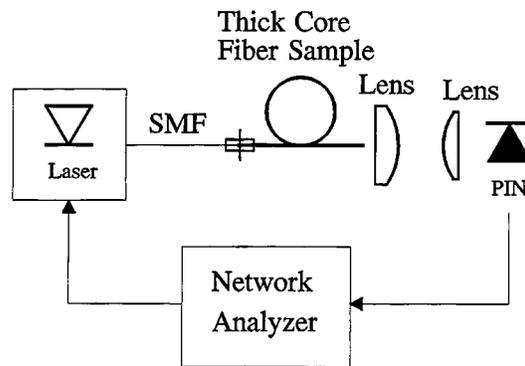
Fig. 18. Bandwidth measurement setup with network analyzer.
