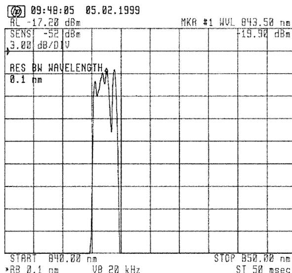
Fig. 11. Optical spectrum of modulated 840-nm VCSEL.
