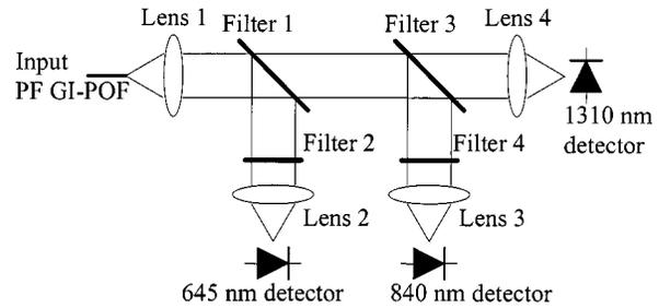
Fig. 14. Principle of operation of the 645-, 840-, 1310-nm demultiplexer.
