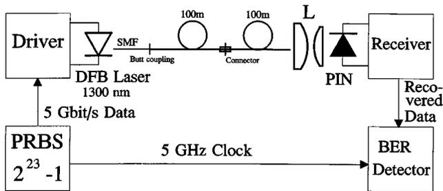
Fig. 13. 5 Gb/s over 200-m PF GIPOF set up.
