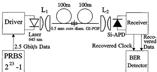
Fig. 4. 2.5-Gb/s transmission over 200 m of PMMA GI-POF.
