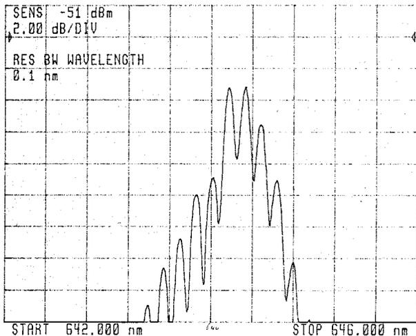
Fig. 7. Measured optical spectrum of the modulated laser.
