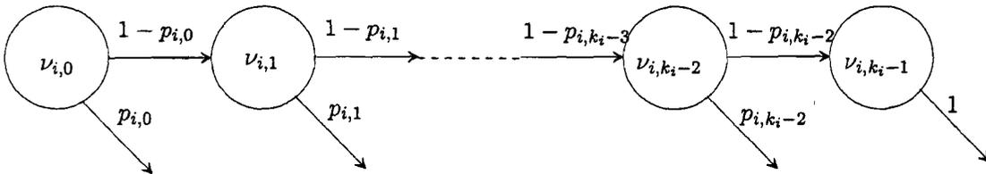
Figure 1: A phase diagram of the Coxian distribution of the inter-arrival time of the  $i$ -th arrival process.
