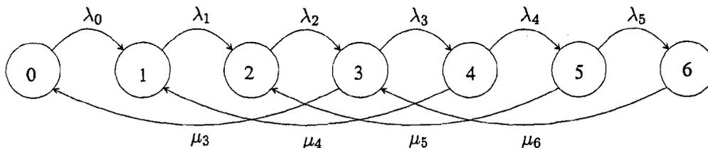
Figure 3: A diagram of the aggregated MAP of the superposition of two Erlang<sub>4</sub> arrival processes.
