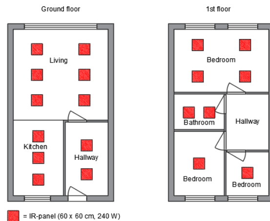
Figure 52: Overview of the placement of the infrared panels in each room of the high insulation terraced house
