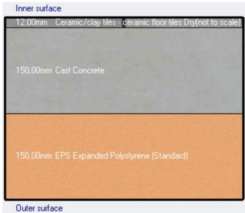
Figure 49: Detail of the ground floor of both houses in DesignBuilder (high insulation)
