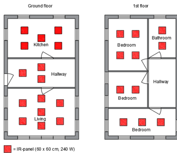
Figure 54: Overview of the placement of the infrared panels in the high insulation freestanding house
