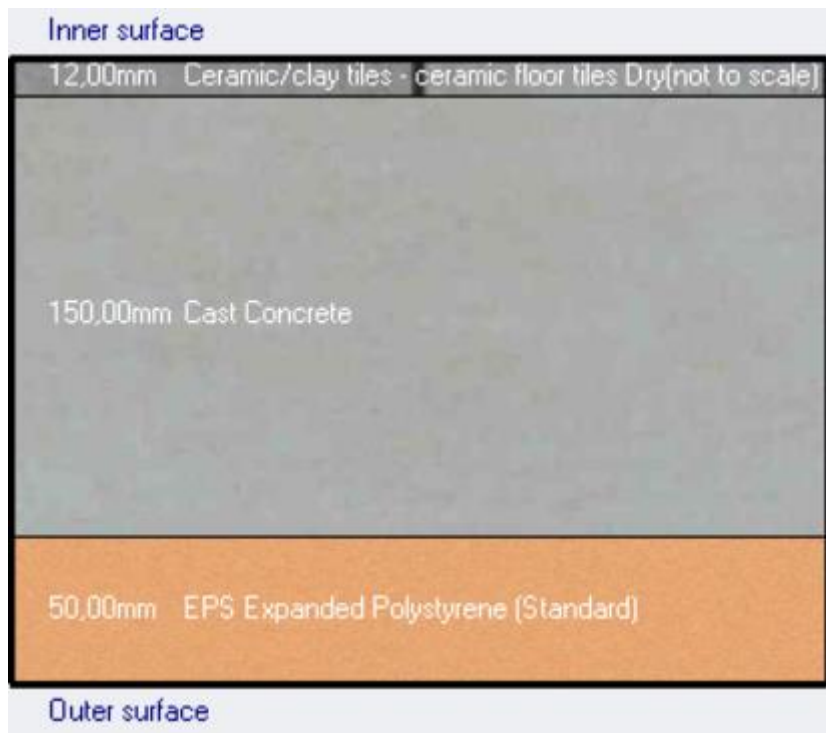
Figure 43: Detail of the ground floor of the terraced house in DesignBuilder (low insulation)
