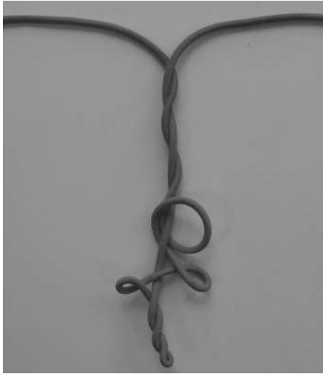
Figure 1.5: A rod configuration that is not a global minimizer, but only a local minimizer. Such configurations are quite stable under perturbation and geometrically diverse, indicating that minimizing elastic energy among all free rods poses a significant challenge.
