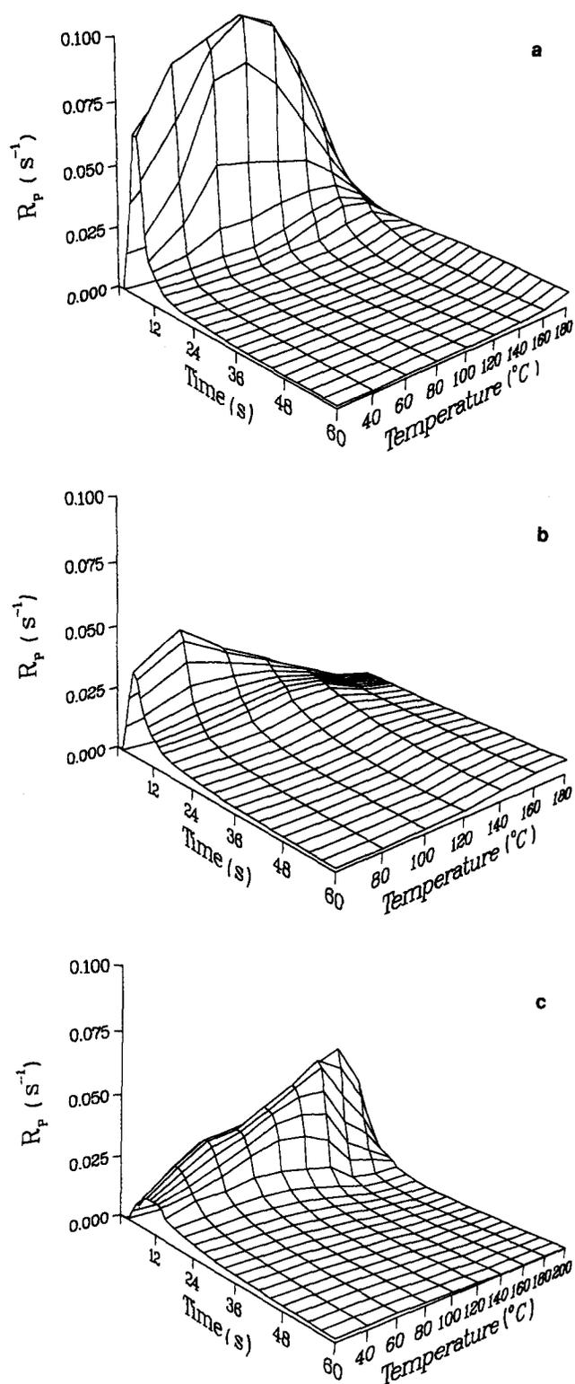
**Figure 2** Polymerization rate in moles C=C bonds converted per second, normalized to the initial C=C bonds concentration, as a function of time and temperature of (a) diacrylate 1, (b) diacrylate 2 and (c) dimethacrylate 3
