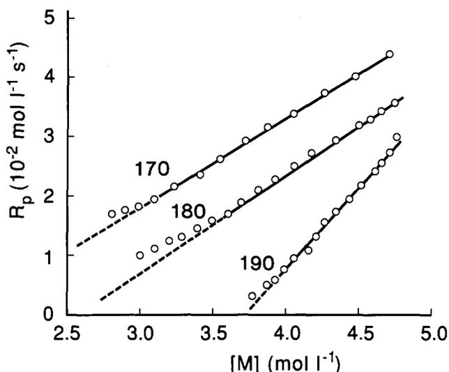
Figure 6 Polymerization rate of diacrylate 2 as a function of the monomer concentration during the course of the photopolymerization at the indicated temperatures (°C)
