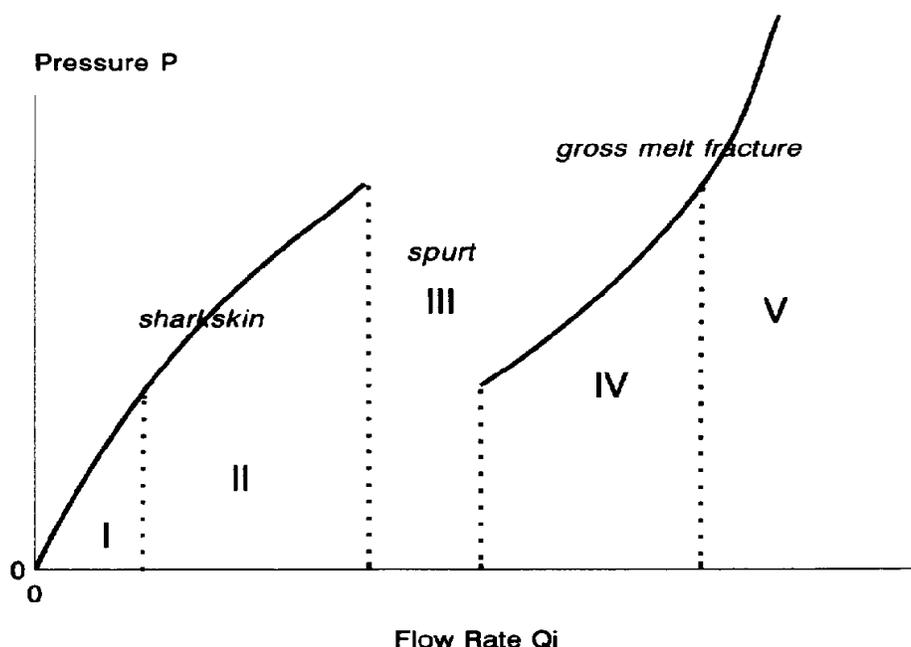
**FIG. 1.** A graphical representation of a typical relation between pressure in the barrel and the flow rate of the extrudate for a capillary rheometer experiment. The four different flow regimes identified as I, II, III are associated with the occurrence of different types of extrudate distortions, i.e., steady state, "sharkskin," "spurt," and melt fracture, respectively. Regimes IV and V are associated with the occurrence of various types of "gross" melt fracture.
