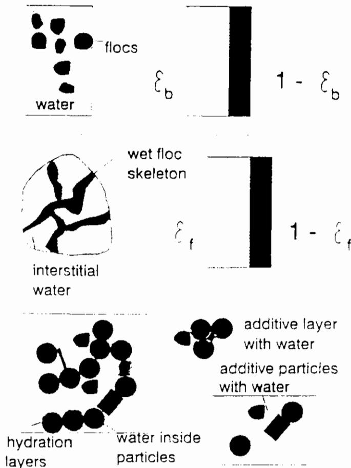
Fig. 1 Schematic representation of water in sludge
