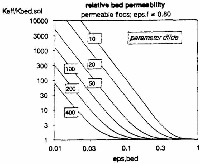
Fig. 5 Relative permeability of porous floc bed  $K_{eff}$  compared to closed particles  $K_{bed,sol}$ , as a function of bed porosity  $\epsilon_{s,bed}$  with relative floc size  $d_f/d_e$  as parameter;  $d_f$  = floc diameter,  $d_e$  = diameter of elementary floc particles. Floc porosity  $\epsilon_{s,floc} = 0.80$ .
