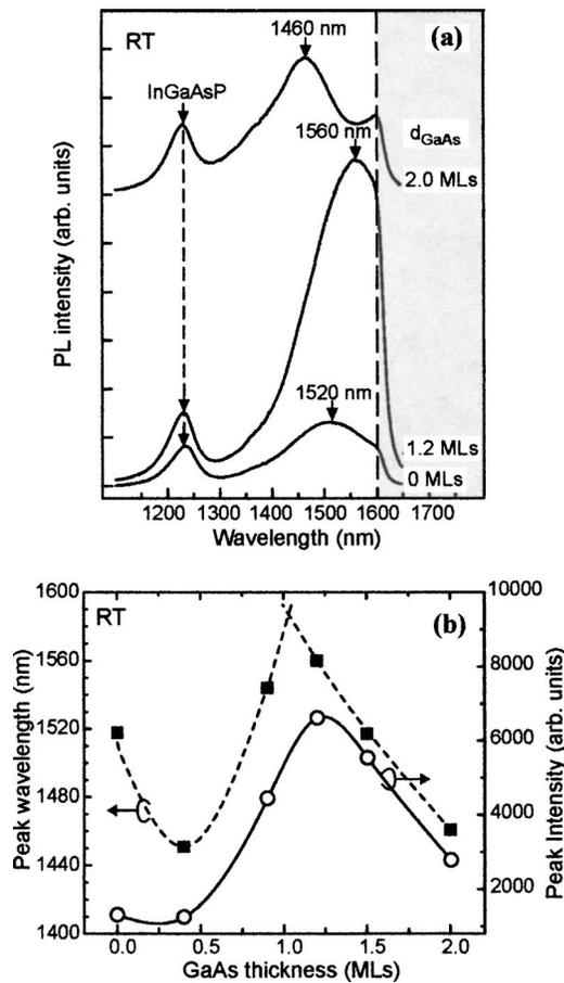
FIG. 6. (a) Room-temperature (RT) PL spectra of the three-MLs InAs QDs of structure B with GaAs interlayer thickness between zero and two MLs. The shaded area is above the detection limit of the cooled InGaAs detector at  $1.6 \mu\text{m}$ . (b) Dependence of the PL peak wavelength and PL peak intensity of the InAs QDs on the GaAs interlayer thickness. The TBA flow rate is  $1.0 \text{ SCCM}$ .
