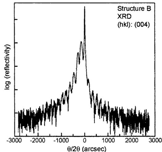
FIG. 3. XRD spectrum of a typical structure B recorded in the vicinity of the symmetric (004) reflection. The three-MLs InAs QDs embedded in an InGaAsP matrix with two-MLs GaAs interlayer are grown at 500 °C.
