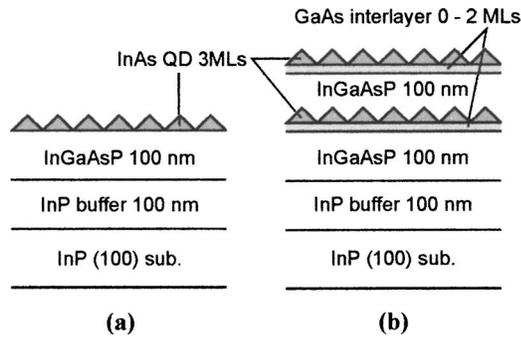
FIG. 1. (a) Sample structure A and (b) sample structure B.
