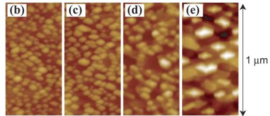
FIG. 2. (Color online) (a) QD height and base diameter as a function of growth temperature. (b)–(e) AFM images ( $0.5 \times 1.0 \mu\text{m}^2$ ) of the QDs of structure A grown at (b) 480, (c) 500, (d) 520, and (e)  $585^\circ\text{C}$ . The height contrast is 40 nm in all images.
