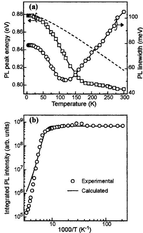
FIG. 8. (a) Temperature dependence of the PL peak energy and PL linewidth of the three-MLs InAs QDs with 1.2-MLs GaAs interlayer. The dashed line is the temperature dependence of the InAs band-gap energy according to the Varshni law, assuming  $E_g=0.88$  eV at  $T=0$  K. (b) Integrated PL intensity of the InAs QDs as a function of temperature. The solid line is the exponential fit with a thermal activation energy of 145 meV.
