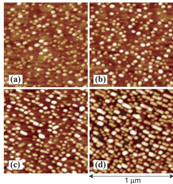
FIG. 7. (Color online) AFM images ( $1.0 \times 1.0 \mu\text{m}^2$ ) of the three-MLs InAs QDs on the surface of structure B with GaAs interlayer thickness of (a) 2.0, (b) 1.2, (c) 0.4, and (d) 0 MLs. The TBA flow rate is  $1.0 \text{ SCCM}$ . The height contrast is  $10 \text{ nm}$  in all images.
