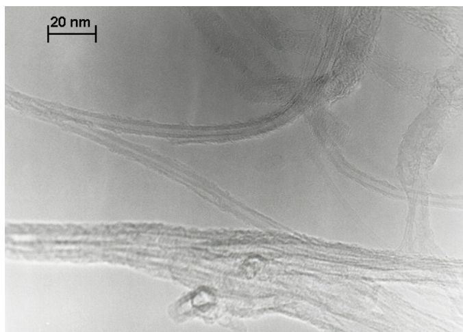
Fig. 91: TEM photograph of a purified MWNT sample ( IMRE ). The MWNTs in this sample consist of a hollow core about 4 nm in diameter and up to 10 walls. The tubes depicted are mostly quite clean (top), but sometimes heavily coated with carbonaceous impurities (bottom).
