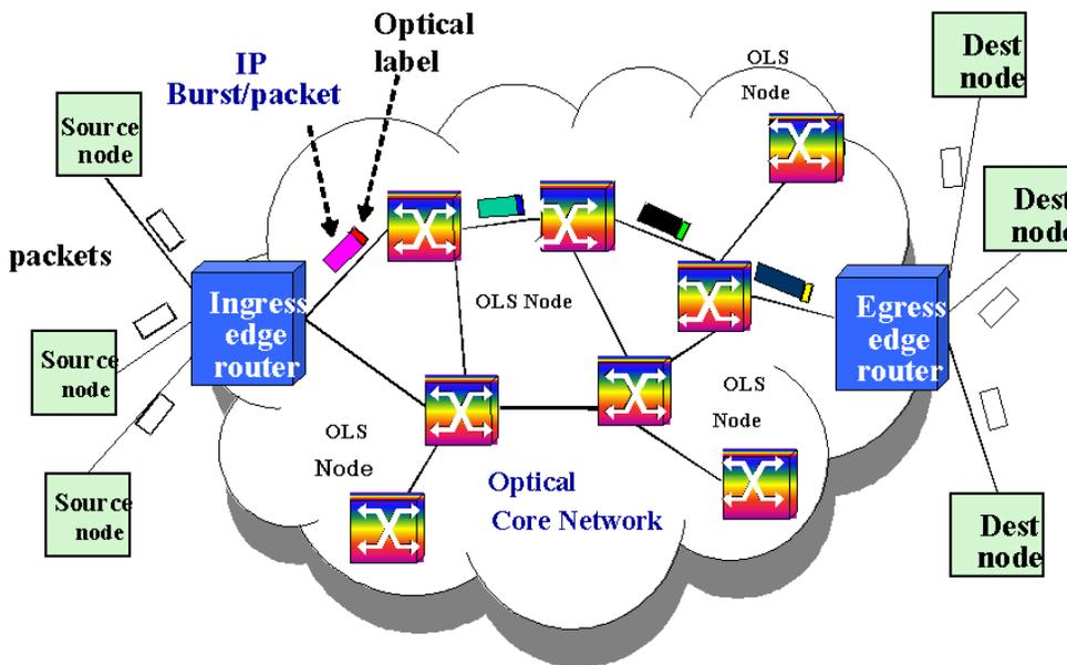
Fig. 1. General overview of the Optical Label Switching (OLS) network architecture.
