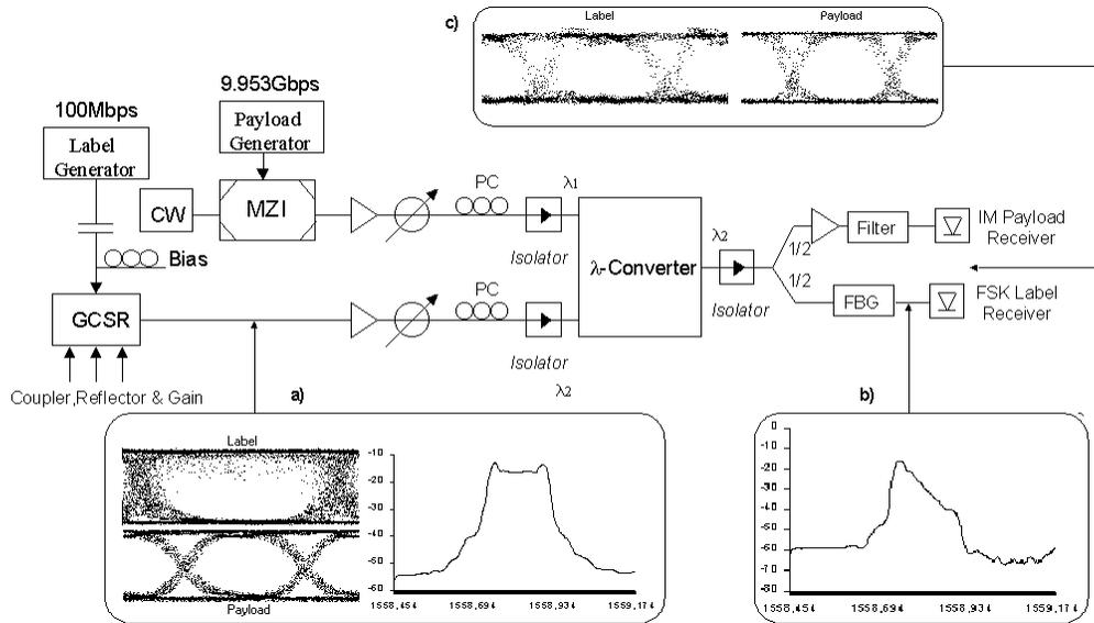
Fig. 3. The experimental setup for FSK/IM generation and label insertion (a), where we can observe the recovered FSK signal (b) and the recovered eye patterns (c).
