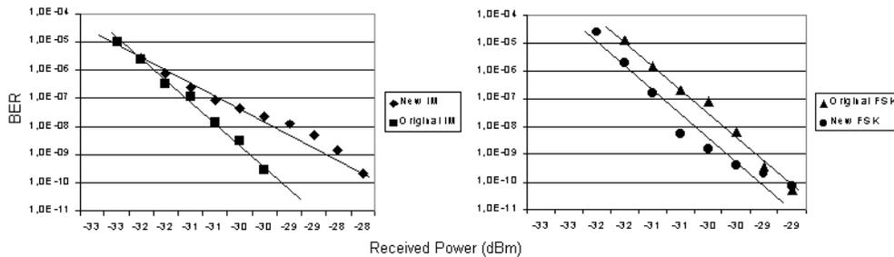
Fig. 4. Comparison of the BER versus the receiver sensibility for the FSK and the IM signal after and before the wavelength converter.
