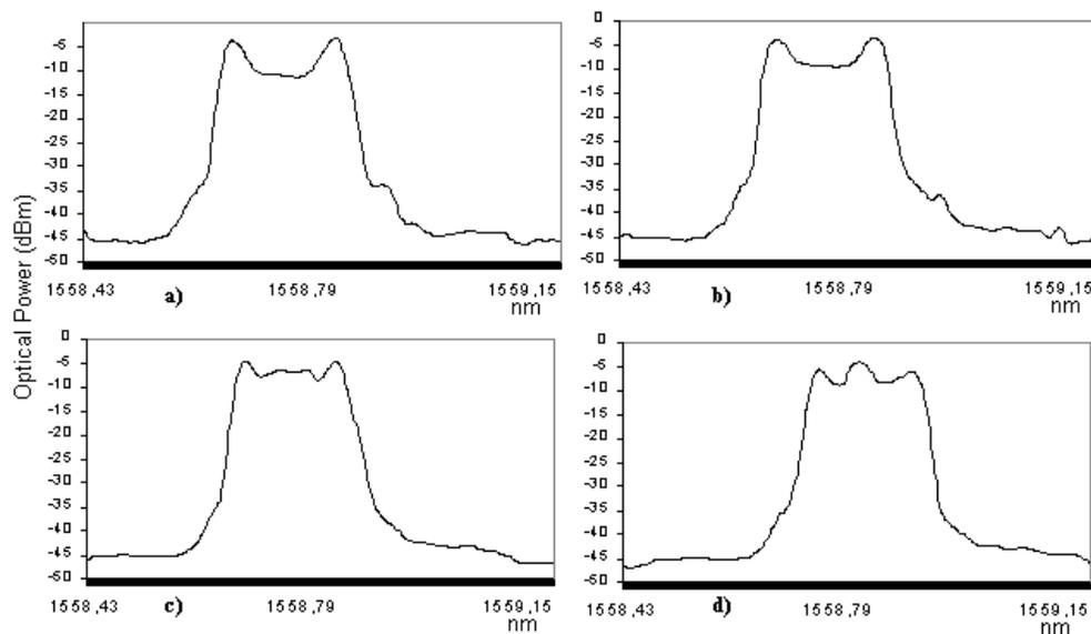
Fig. 2. FSK optical signal with a modulation rate of 50 Mbit/s (a), 78 Mbit/s (b), 120 Mbit/s (c) and 155 Mbit/s (d).
