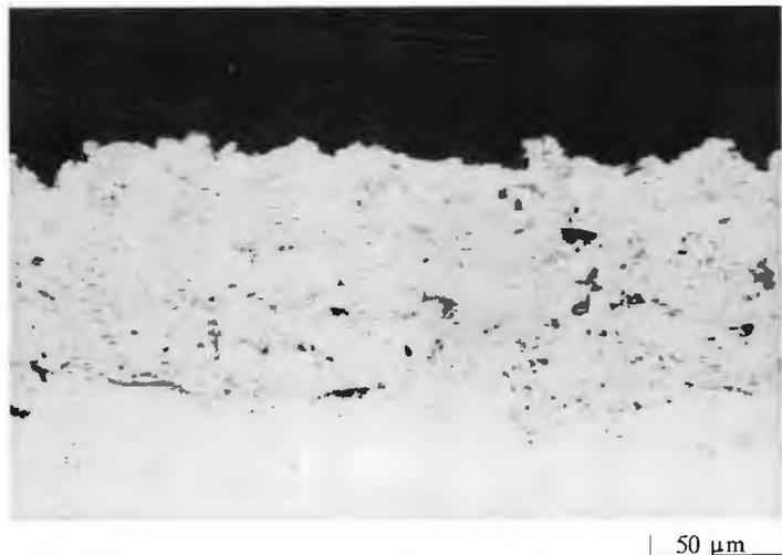
**Figure 3.21** Cross section of a LPPS FeCrAlY bondcoat. The coating shows some pores but no oxides.
