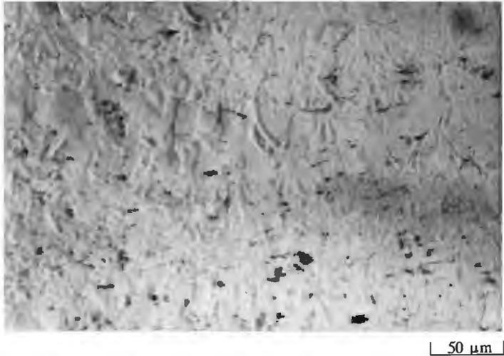
**Figure 3.28** Cross section of a ZrO<sub>2</sub> coating, sprayed with a 120 mm extended anode channel. The boundaries between the individual particles disappeared. A columnar grain structure can be observed.
