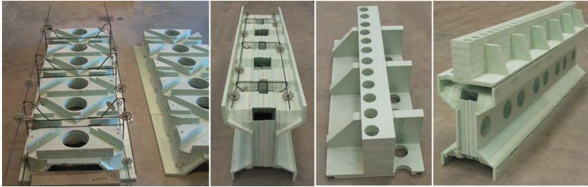
**Figure 3: Three-dimensional shell and edge form**
