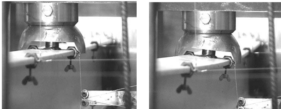
Figure 39: Functioning of the spherical bearing (left before testing, right during testing)
