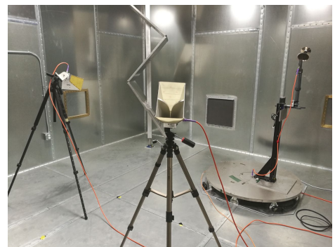
Fig. 4. Setup in the NIST RC. Due to the height of the chamber, the horizontal paddle is not visible in this picture, but it is situated on the top left.
