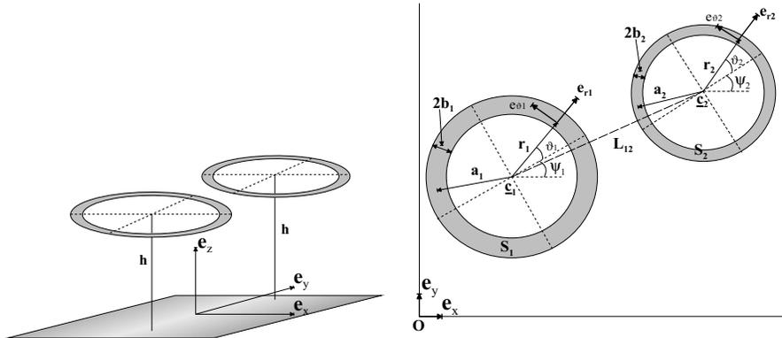
Fig. 1. Geometry of an array of two rings.
