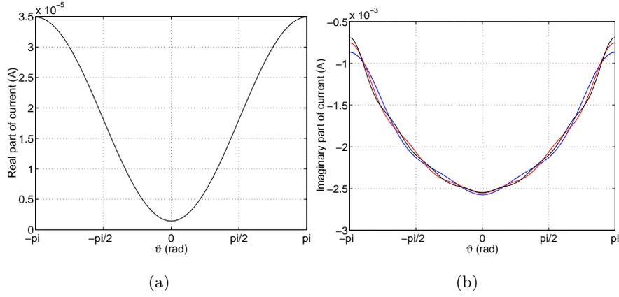
**Fig. 2.** The total current on a ring excited by a voltage gap of 1 V at a frequency of 3 GHz.;  $a = 0.0637\lambda$ ,  $b = 0.0027\lambda$ ,  $\mathbf{c} = (0, 0, 0)$ , and  $\psi = 0$ . (a) Real part; 2 expansion functions of cosine type. (b) Imaginary part; blue, red, black: 4, 6, and 8 expansion functions of cosine type.
