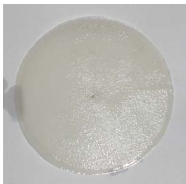
Figure 7: A used nanofiltration membrane (Koch MPF-50).
