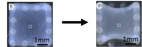
Figure 3: manipulation of mechanical constraints to induce anisotropic cell organization and matrix remodeling. Obbink-Huizer et al., Biom Mod Mech , 2014.
