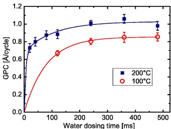
**Figure 3.** (Color online) GPC of thermal ALD Al<sub>2</sub>O<sub>3</sub> as a function of water dosing time. Data is given for substrate temperatures of 100 and 200°C. The lines serve as a guide to the eye.
