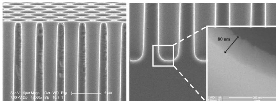
**Figure 6.** High-resolution SEM images of Al<sub>2</sub>O<sub>3</sub> deposited by remote plasma ALD in macropore structures with an aspect ratio of ~8 (diam: 2–2.5 μm, depth: 19 μm). The Al<sub>2</sub>O<sub>3</sub> was deposited using 700 ALD cycles.
