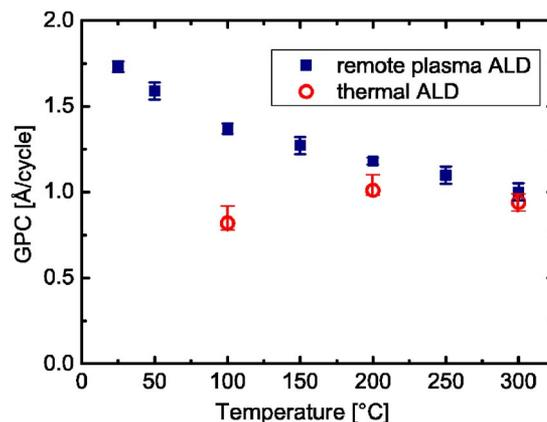
**Figure 4.** (Color online) GPC of Al<sub>2</sub>O<sub>3</sub> as a function of substrate temperature for remote plasma and thermal ALD.
