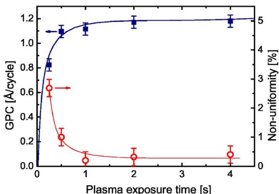
**Figure 2.** (Color online) The growth per cycle (GPC) and nonuniformity for remote plasma ALD Al<sub>2</sub>O<sub>3</sub> as a function of plasma exposure time. The nonuniformity was determined over a 150 mm wafer. The substrate temperature was 200°C and a 400 W plasma power was used. The lines serve as a guide to the eye.
