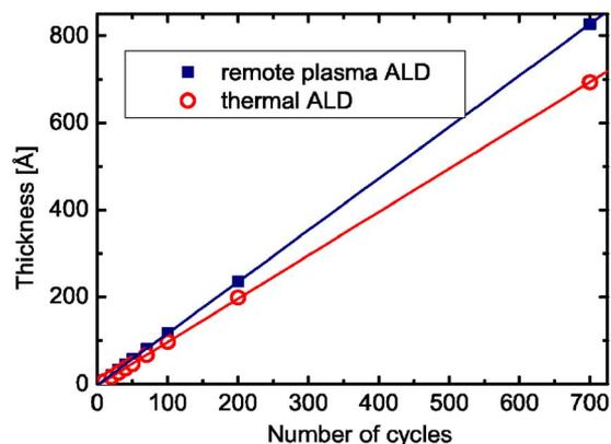
**Figure 1.** (Color online) Al<sub>2</sub>O<sub>3</sub> film thickness as a function of the number of cycles for both remote plasma ALD and thermal ALD. The thickness was determined by in situ spectroscopic ellipsometry and the growth per cycle was obtained from the linear fits shown in the figure. The substrate temperature was 200°C.
