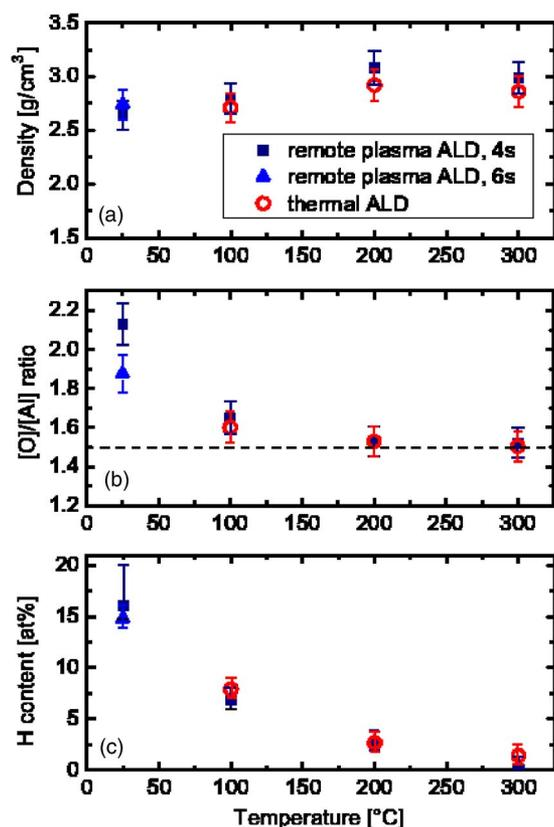
**Figure 5.** (Color online) Material composition as a function of substrate temperature. (a) Mass density as determined from RBS and ellipsometry. (b) [O]/[Al] ratio as determined from RBS. (c) H content as determined by elastic recoil detection. For the deposition at 25°C, data is given for both the standard recipe (4 s cycle time, 2 s plasma exposure) and for extended plasma exposure (6 s cycle time, 4 s plasma exposure).
