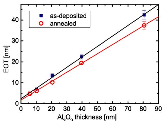
**Figure 7.** (Color online) EOT vs physical thickness of Al<sub>2</sub>O<sub>3</sub> films deposited at 200°C by remote plasma ALD. Results for both the as-deposited and the annealed (425°C, forming gas) material are shown.
