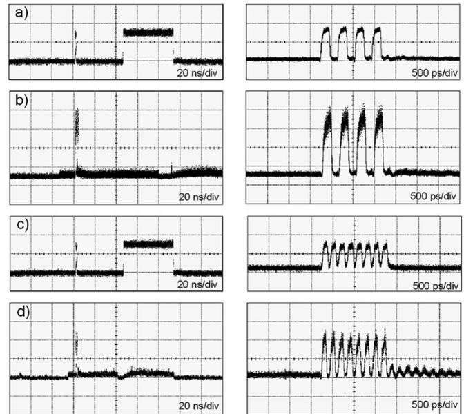
Fig. 4. Traces of the label separation for a bit rate of 5 and 10 Gb/s. (a) and (c) correspond to the burst and its label at 5 and 10 Gb/s, respectively. (b) and (d) correspond to the separated label and a detail of the separated label at 5 and 10 Gb/s, respectively. The vertical axis scale is 5 mV/div in all the pictures.
