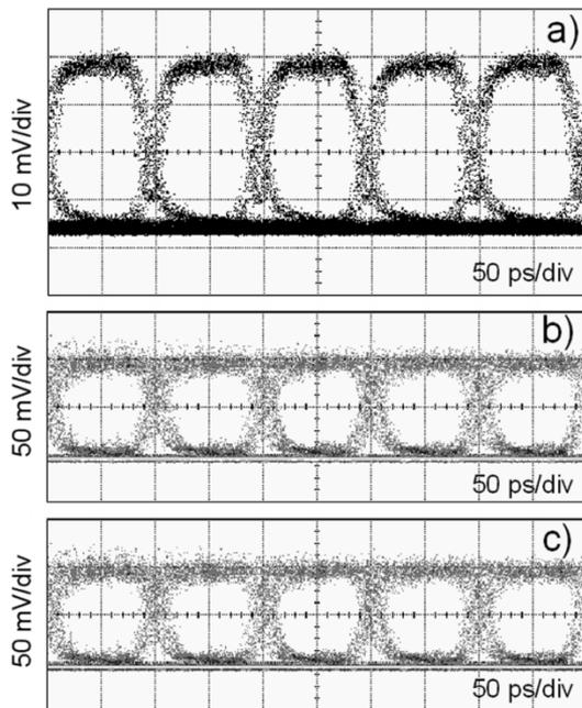
Fig. 6. Eye diagrams of (a) the original payload signal, (b) the separated short payload, and (c) the separated long payload.
