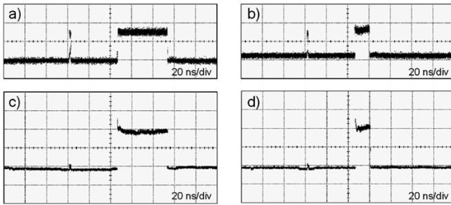
Fig. 5. Traces of the original burst with (a) a long and (b) a short payload for a 10-Gb/s label, and (c), (d) the output of the payload port, where we obtain only the payload. The vertical axis scale is 5 mV/div in all the pictures.
