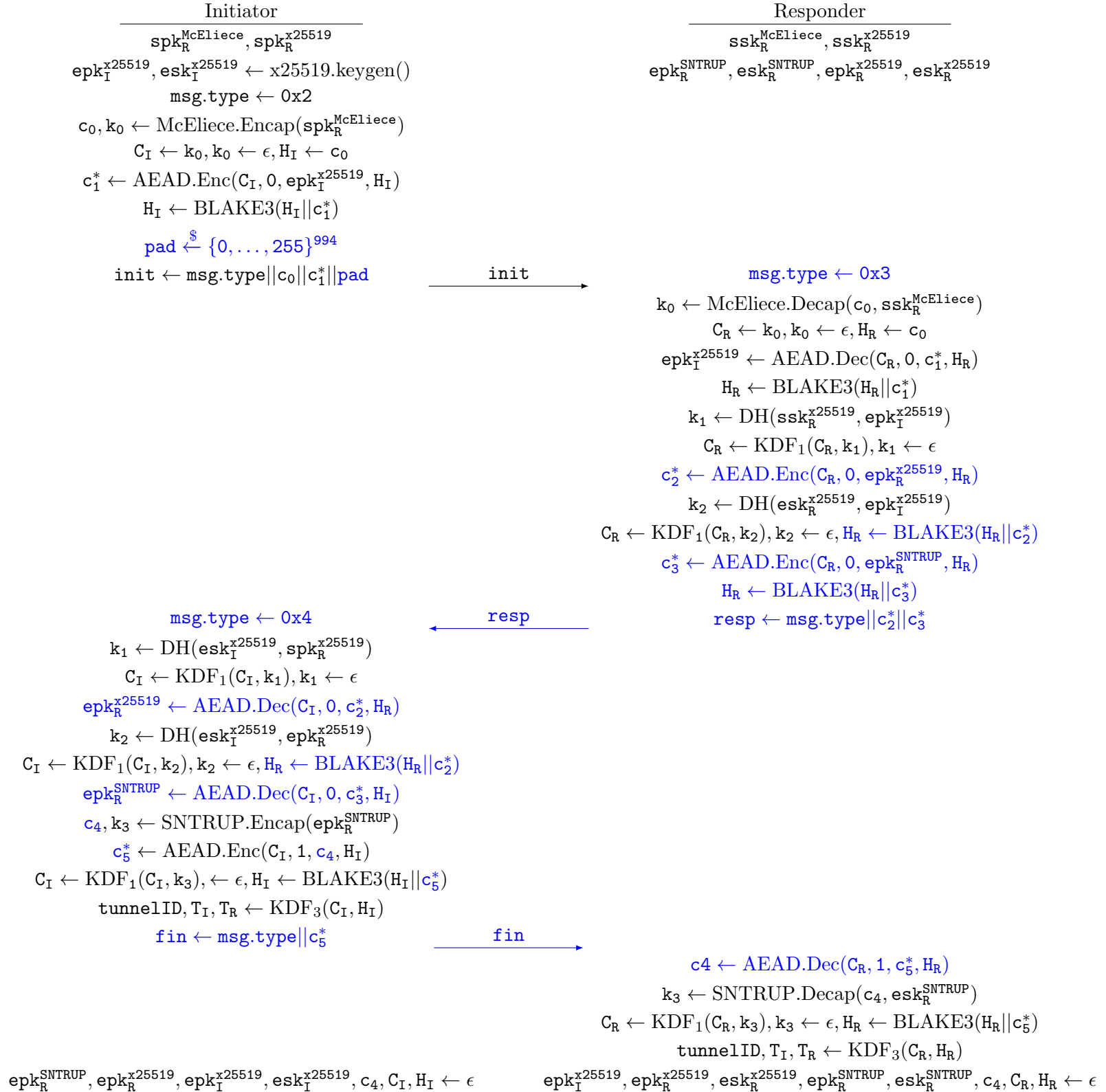
Figure 3.3: A first attempt at a 1-RTT PQConnect Handshake if the Initiator does not know the Responder's ephemeral keys. Differences from Figure 3.2 are highlighted in blue.
