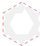
Figure 2.33: Silhouette of a strip which does not have a crease on the convex hull. Unfolding any crease will make the silhouette fold within its own convex hull.
