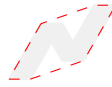
Figure 2.32: A small example of a silhouette which does not have a crease on the convex hull. The convex hull is made to be axis aligned, as this is the only lines which are interesting for our problem.
