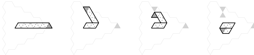
Figure 2.4: Example of a strip folding to different locations. The maximum reachable locations are indicated by the border around the strip. The previous locations are also marked.
